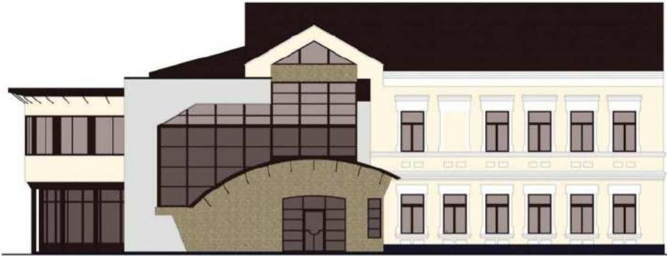
Reconstruction design of Daugavpils branch of Baltic Transit Bank included replacement of roof structure for existing building, construction of new structure and landscaping works.
